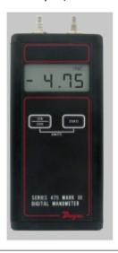
The Series 475 Intrinsically Safe Handheld Digital Manometer measures positive, negative, or differential pressures of air and natural gases in ranges from 1 in w.c. (0.249 kPa) to 150 psid (10.34 bar). The dual push pads on the front panel control the on/off, auto zero, and pressure unit selection, allowing for simple operation with no set up needed. When used with a Dwyer® Pitot tube (1), the Series 475 can also be used as an air velocity gage.
