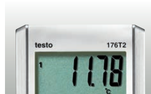
Large, clear display for showing measurement values (testo 176 T2 only)
